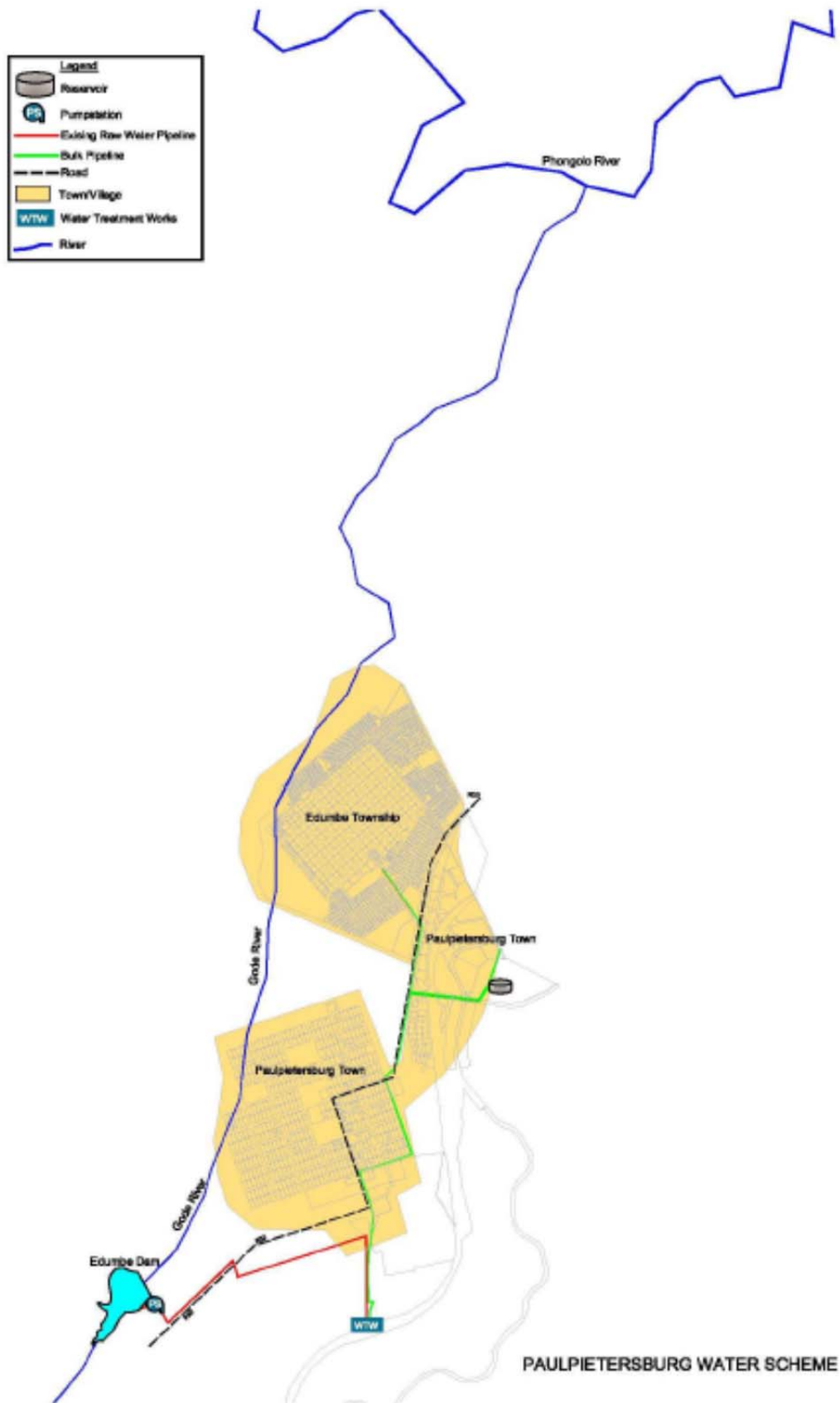
Figure 19 - Schematic layout of Paulpietersburg Water Supply Scheme
