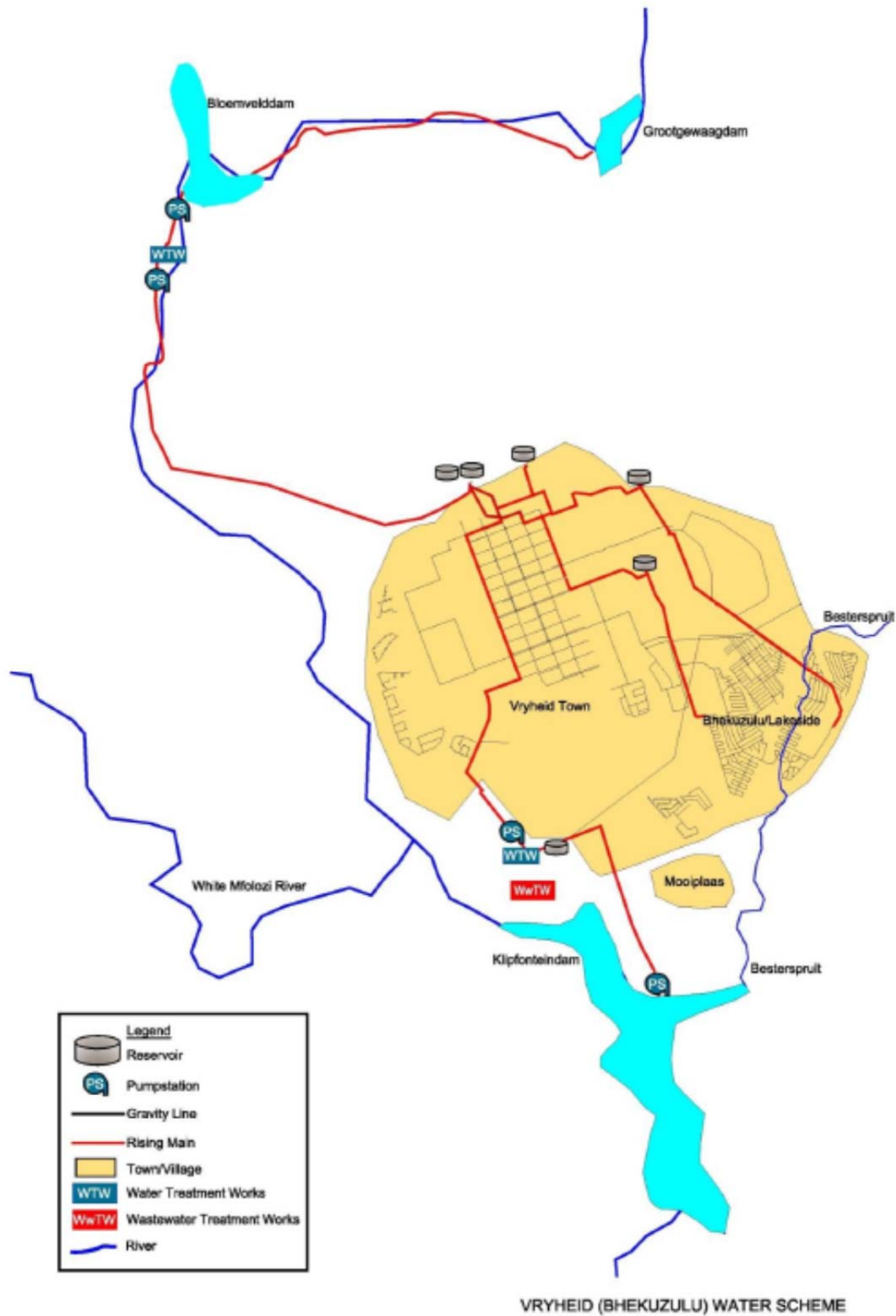
Figure 15 - Schematic layout of Vryheid Water Supply Scheme
