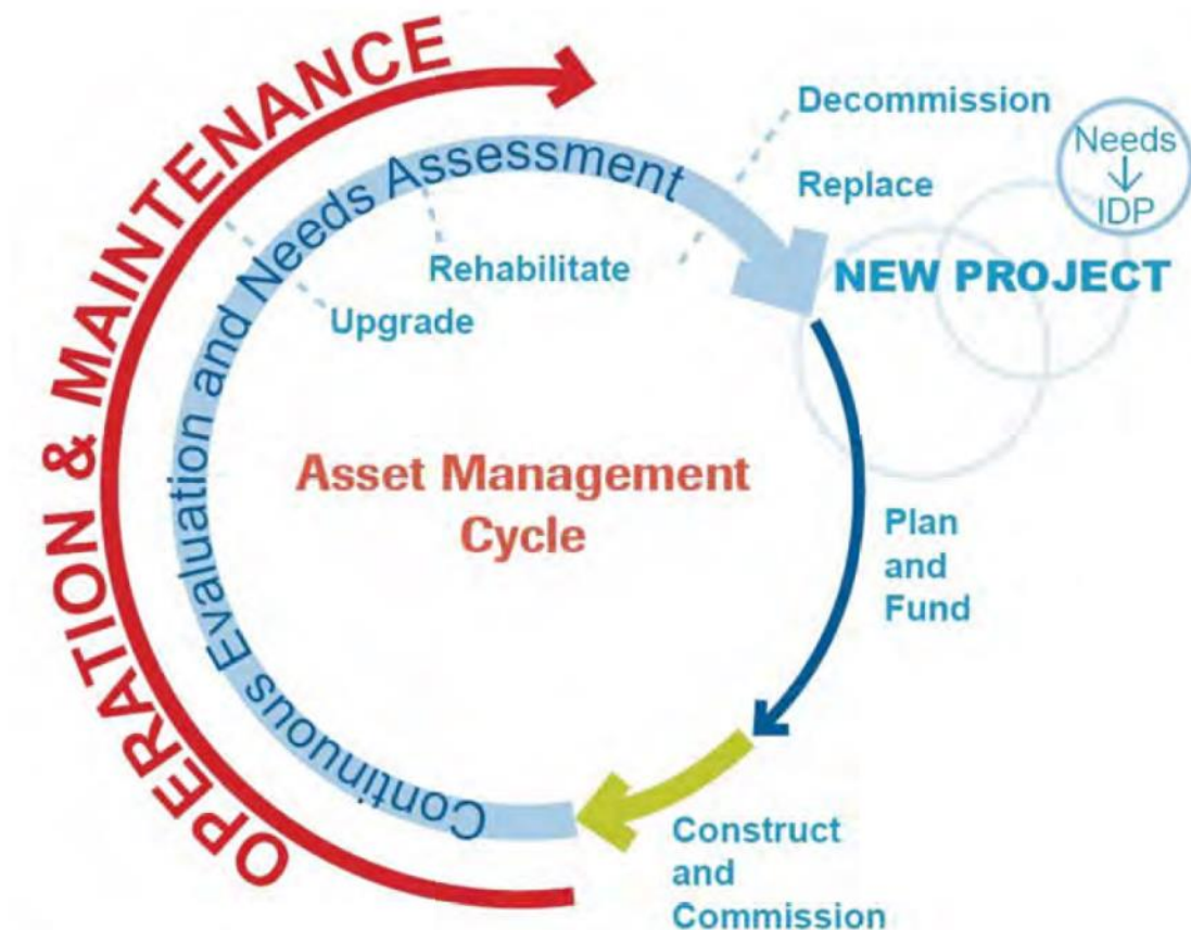
Figure 14.53 Integrated asset management (DWS 2018: 5-14).
