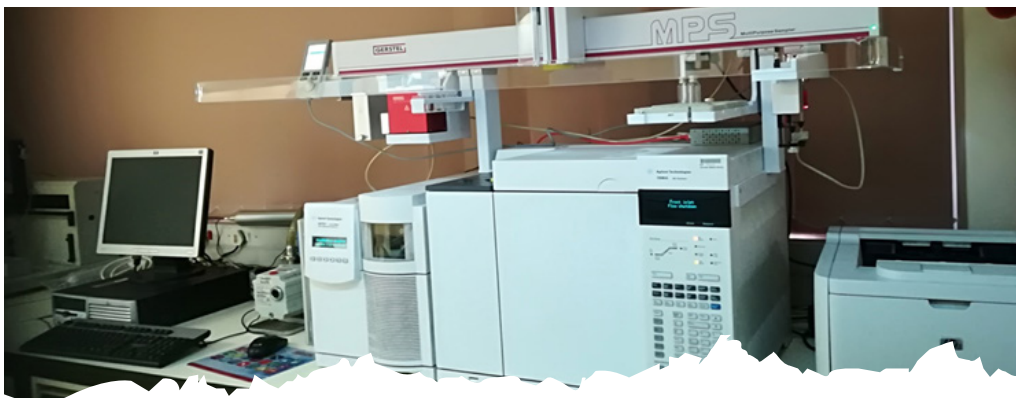
Figure 1: The New GERSTEL Multipurpose Sampler (MPS), Installed onto an Agilent Gas Chromatograph-Mass Spectrometer, at Head Office Laboratory: Chemistry.
