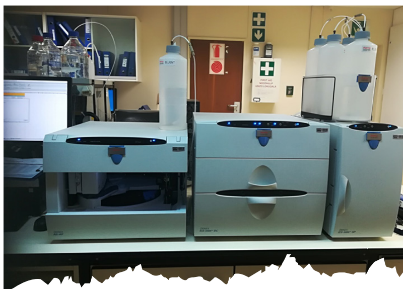
Figure 1: The New Suppressed Ion Chromatograph - Conductivity Detector System at Head Office Laboratory: Chemistry.
